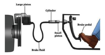
Fig 1.2: Braking System
