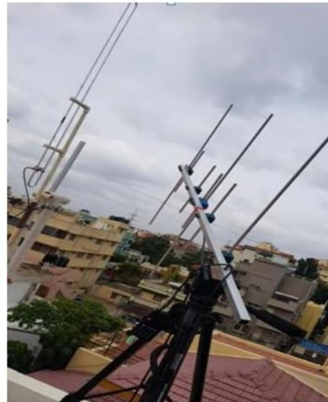
**Figure – 6.21 Yagi u da Antenna Installed in Terrace for real time communication projects**
