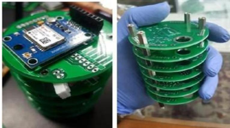
**Figure 6.16- CAN -SAT Communication Module**
